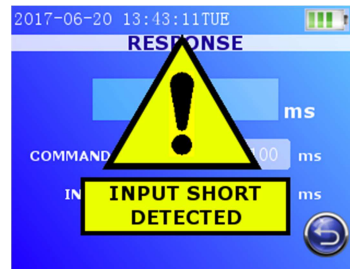
Fig. 10 Result in case of short circuit on input
